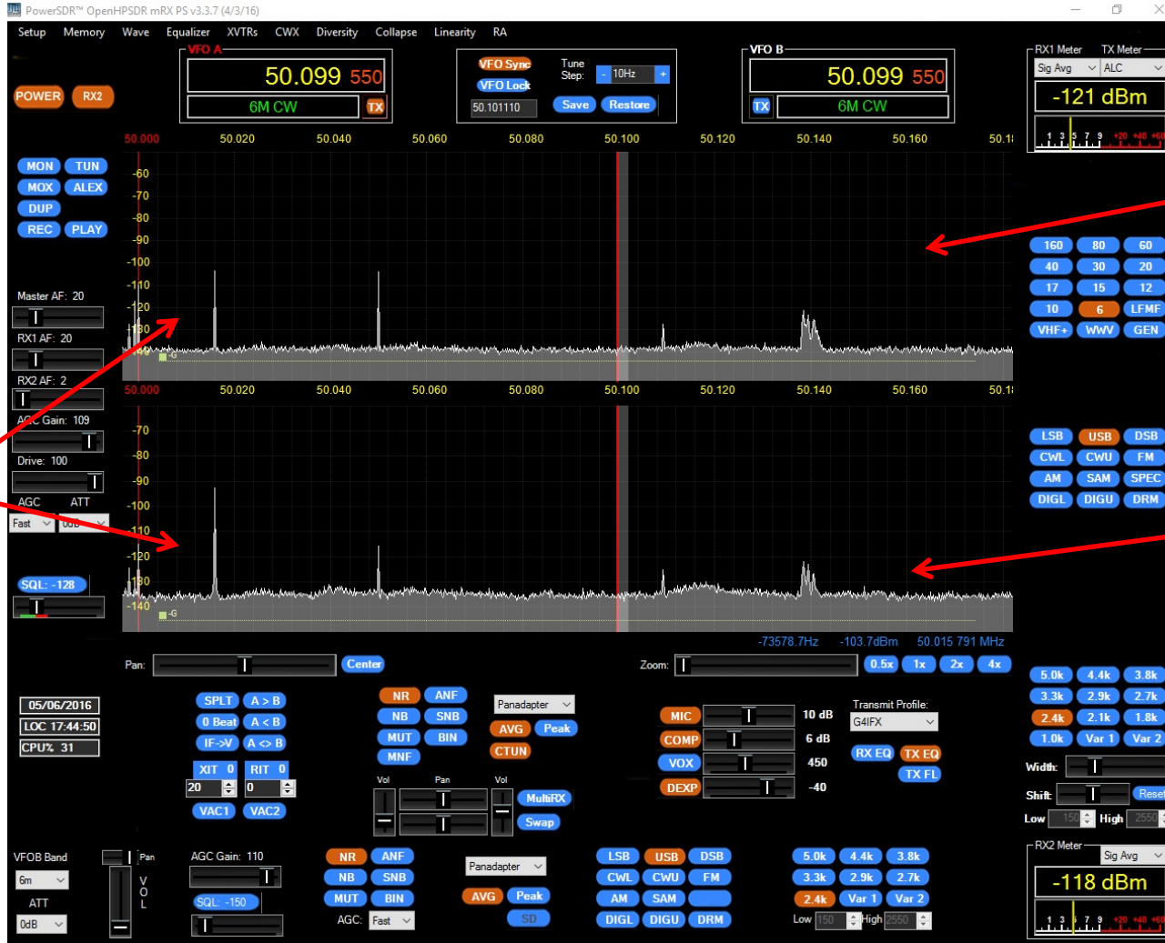
Apache ANAN-100D, dual receivers, OpenHPSDR mRX PS (nearly) identical receiver chains – effectively a dual channel spectrum analyser
